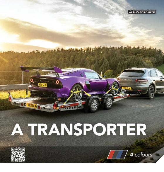
An open car trailer with a 3000kg gross weight, perfectly suited for vehicle recovery, transport logistics and motorsport. A Transporter features easy glide, internally stored ramps and a flush centre deck.
